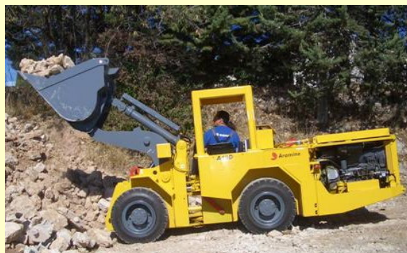
The introduction of narrow mini-scoops (pictured above) are expected to have a favourable impact on development grades
